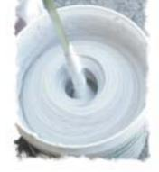
Joint compound consistency is an important part of achieving a good finish. Automatic taping tools require a thinner compound (more water) than setting by hand. The consistency should be smooth and creamy, slightly thinner for taping, slightly thicker for finishing. Ensure you follow manufacturers recommendations.
